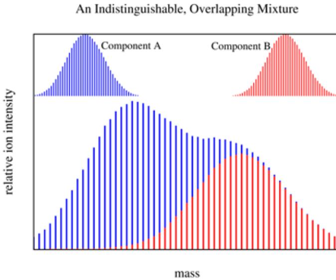
Figure 4— Schematic illustration of an indistinguishable and overlapping mixture of two components, where the peak intensities in the mixture are simply sums of component oligomer intensities.
