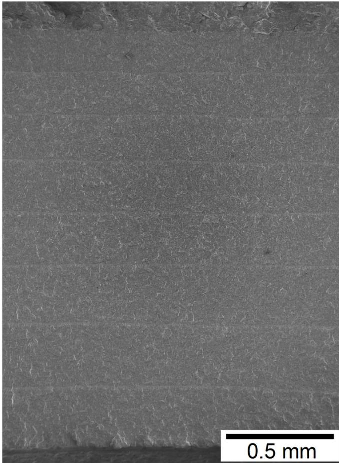
Figure 9 – SEM image of fatigue pre-crack fracture surface showing fatigue marker bands. Initial EDM notch geometry was 5.4 mm deep by 28.3 mm wide.
