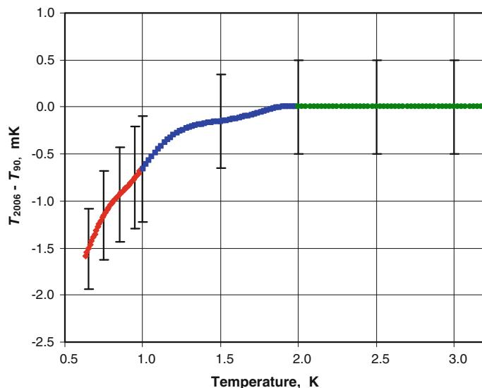
**Fig. 4** Differences between the scales PTB-2006 and ITS-90. The temperature scale PTB 2006 is based on the PLTS-2000 (red symbols, left), on a thermodynamic vapor-pressure relation (blue symbols, middle) and on the ITS-90 (green symbols, right). The error bars represent uncertainties for  $k = 1$  (Color figure online)
