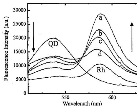
**Figure 1.** Fluorescence spectra of microfluidic channels containing control PEMs with quantum dots or rhodamine and microfluidic channels containing quantum dots and rhodamine, which are separated by 2 (a), 4 (b), 6 (c), and 8 (d) layers of polyelectrolyte layers.
