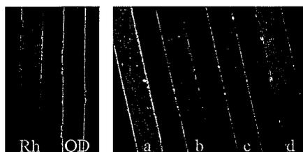
**Figure 2.** Fluorescence images of microfluidic channels (50  $\mu\text{m}$  wide, 30  $\mu\text{m}$  deep, and 3 cm long) containing control PEMs with rhodamine (Rh) or quantum dots (QD) and microfluidic channels containing quantum dots and rhodamine, which are separated by 2 (a), 4 (b), 6 (c), and 8 (d) layers of polyelectrolytes.
