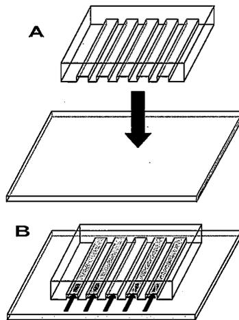
**Preparation of the FRET sensing film using the layer by layer (LbL) deposition method** - . Scheme S2 illustrates the fabrication of PEMs in microfluidic channels by
