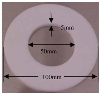
Fig.5 Teflon adapter for 50mm substrate etching
