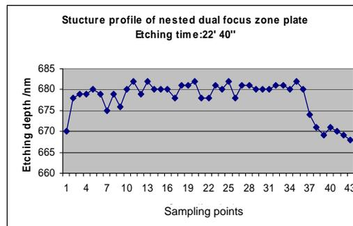
Fig.6 Final part profile by RIE with implementing of Teflon adapter
