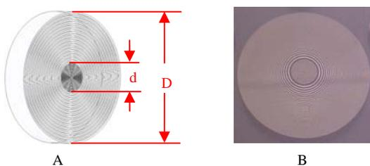
Fig.2 Nested dual-zone pattern; A) pattern Diagram  $d=12.7$  mm,  $D=50$  mm; B) Photo mask of dual-zone zone plate
