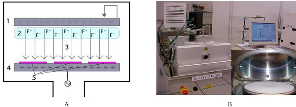
Fig.1 Reactive-ion Etching facility. A) Diagram of a common RIE setup. An RIE consists of two electrodes (1 and 4) that create an electric field (3) meant to accelerate ions (2) toward the surface of the samples (5). B) Picture of commercial RIE
