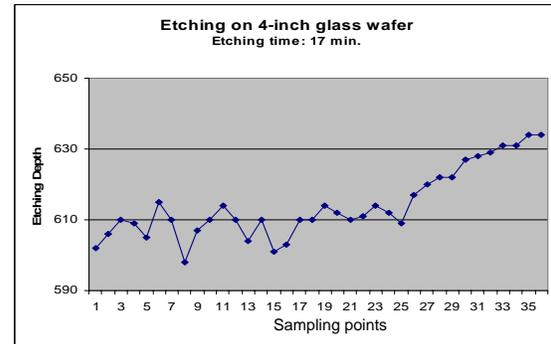
Fig.4 Etching Depth on 4-inch glass wafer
