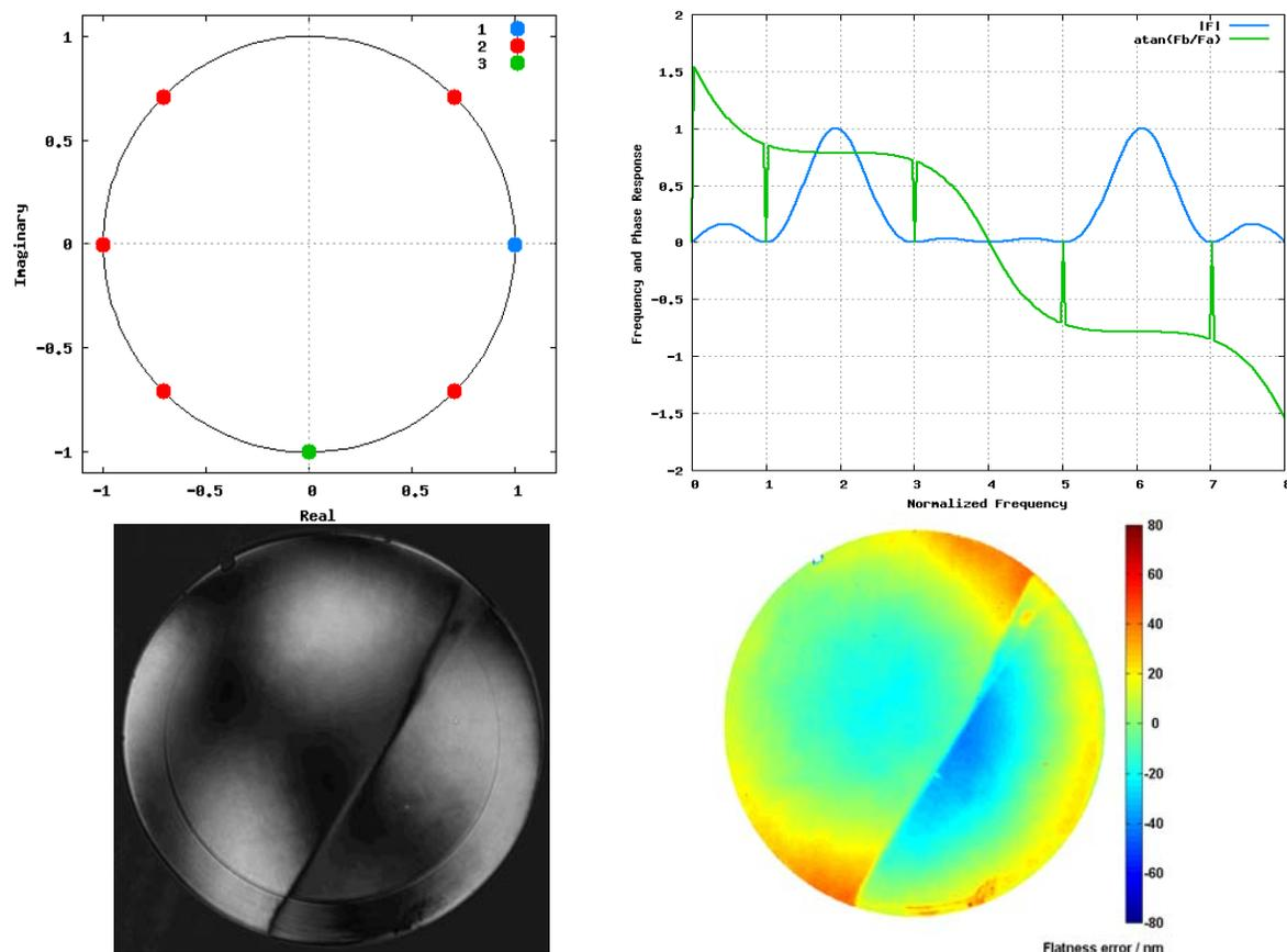
Figure 2: 15-sample, 45° PSA and its spectral response (top row), and fringes and flatness error of the front surface of a plane-parallel window, measured with this PSA (bottom row).
