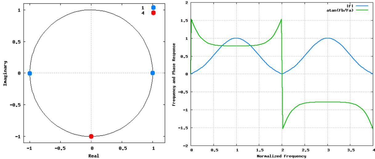
Figure 1: Characteristic diagram (left) and spectral response (right) of the 7-sample, 90° de Groot phase-shifting algorithm.
