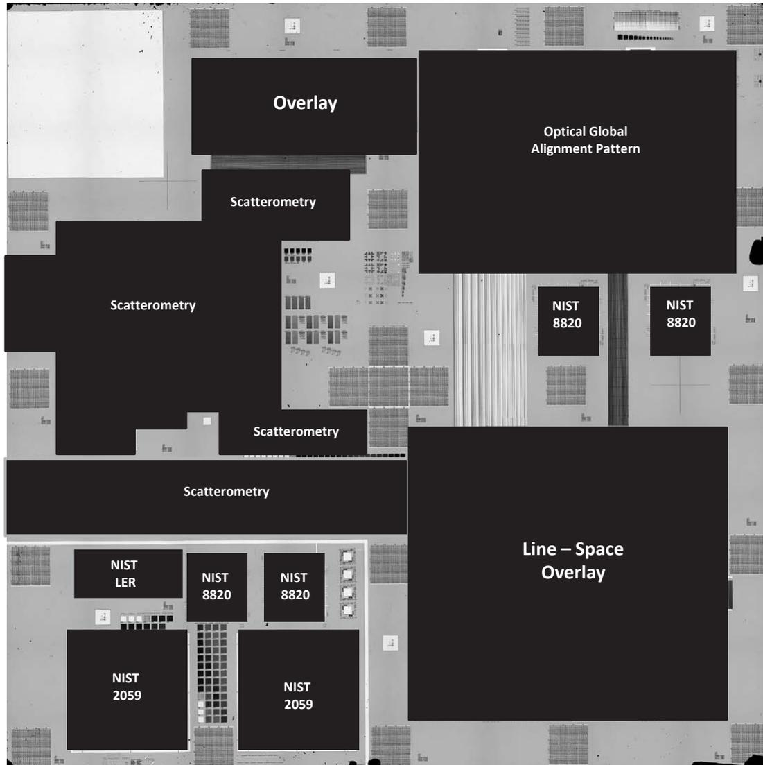
**Figure 2. Identification and highlighting of some of the types of calibration and testing patterns available on RM 8820, overlaid on the bright field optical micrograph of Figure 1.**
