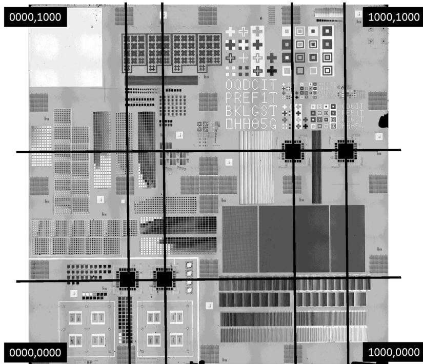
**Figure 3. Optical micrograph of the overall RM 8820 with the global grid applied and the four NIST RM 8820 patterns shown at the coordinate locations described in the text.**
