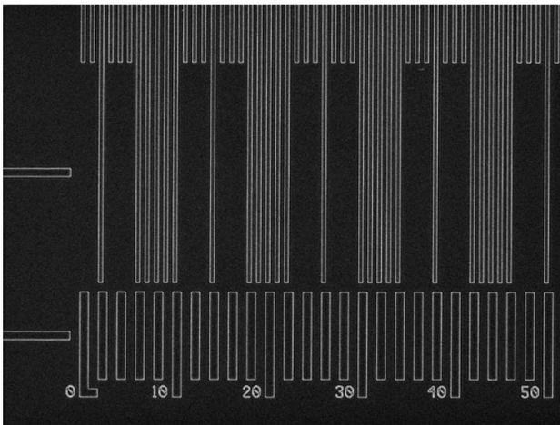
Figure 7. Typical low-magnification image of a roughly 50  $\mu\text{m}$  portion of the binary-type pitch structure. The 2  $\mu\text{m}$  pitch-numbered guiding lines at the bottom and the isolated and dense structures are clearly visible.
