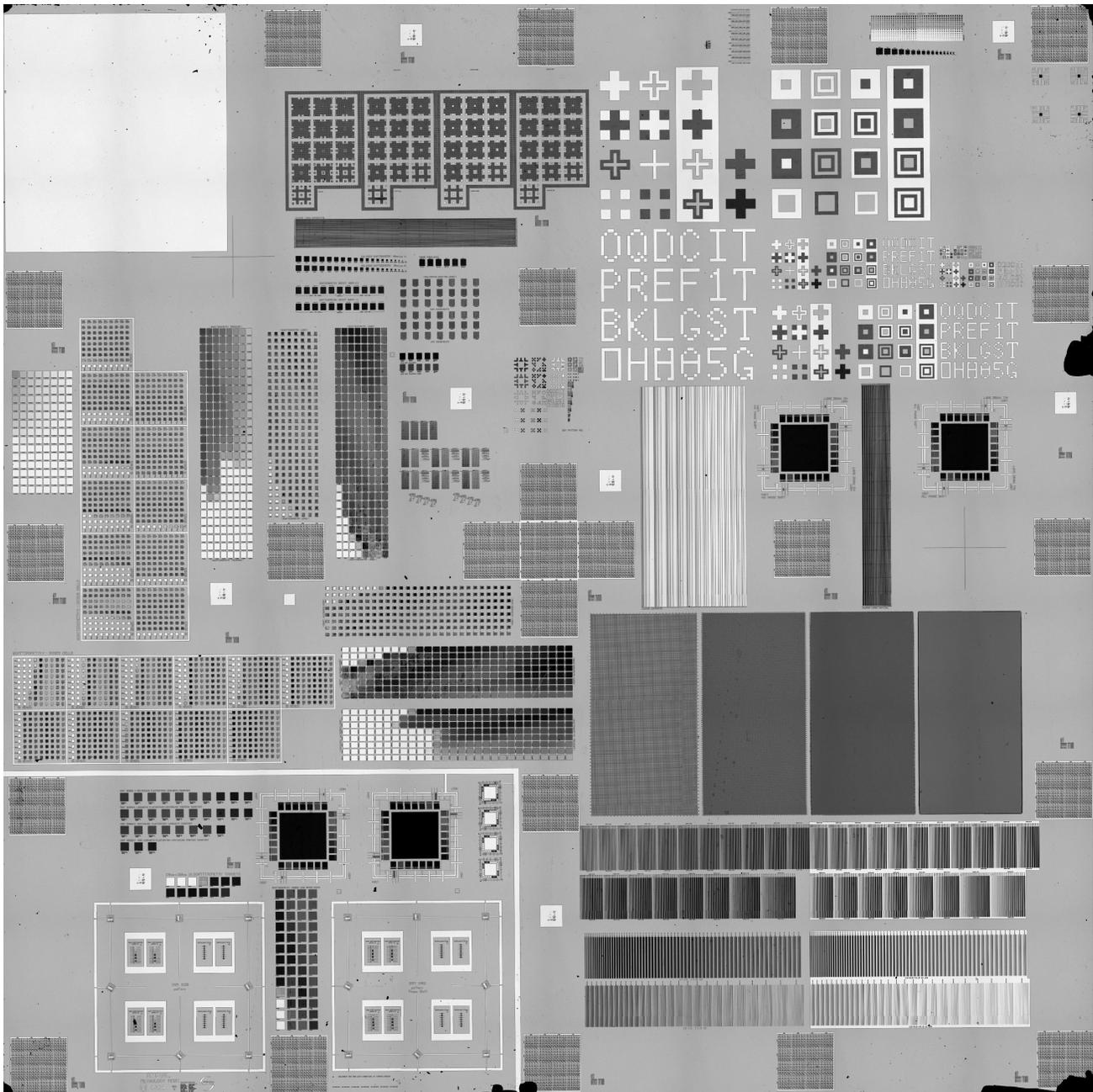
Figure 1. Overall bright field optical micrograph of the RM 8820 sample. (Courtesy of Zeiss, Inc.)
