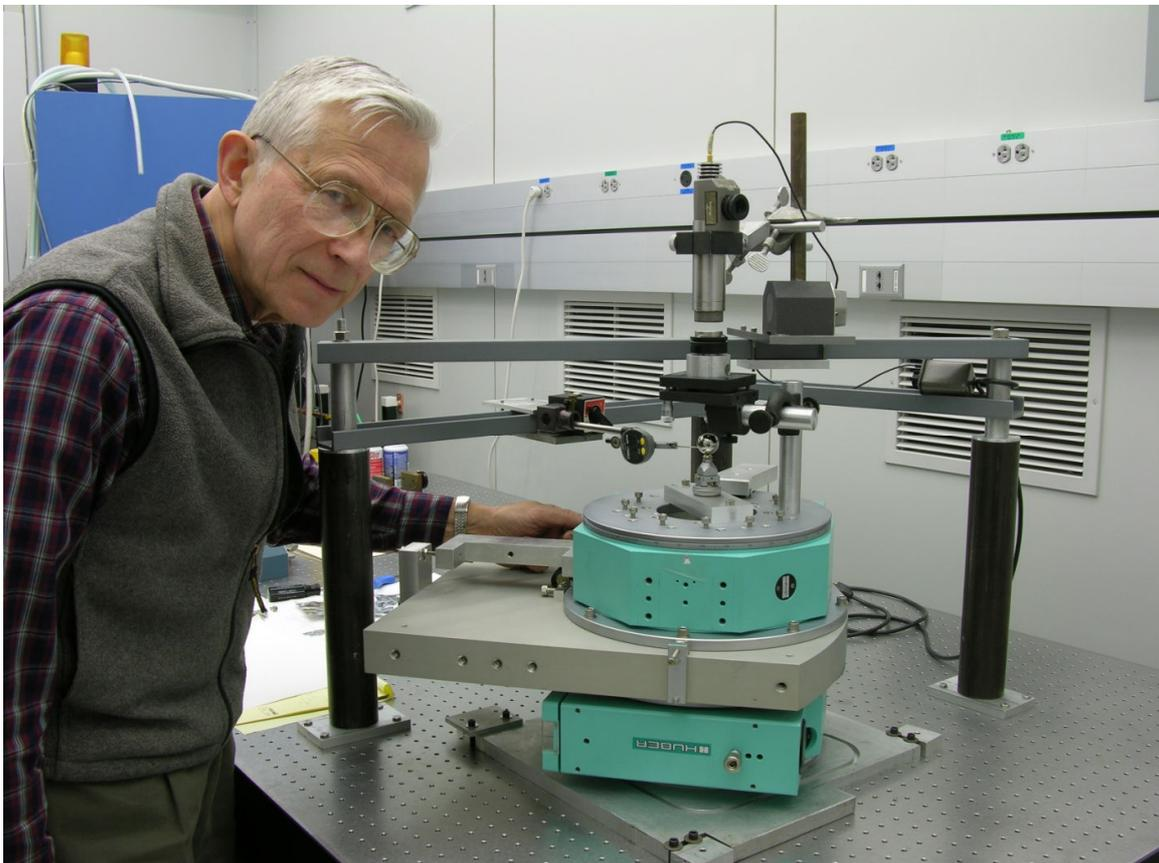
Figure 7. Albert Henins displaying his apparatus for aligning the rotation axes of the CDDBD
