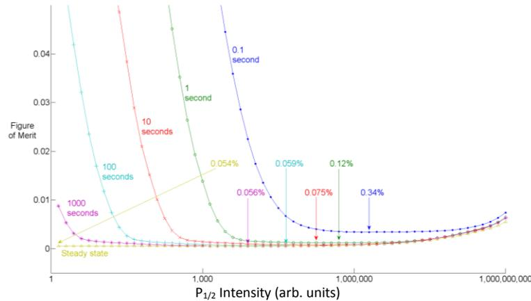
Fig. 2. Figure of merit (which we minimize) vs. intensity in one hole-burning field. Shown are time evolved solutions for five total sequence times (noted) and the steady-state solution. Intensities in the other two fields are optimized at each point. Minima are noted for each curve.
