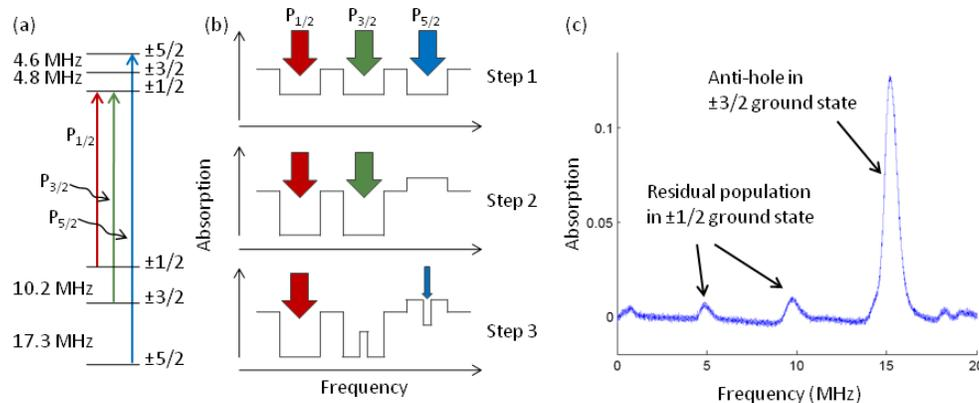
Fig. 1. (a) Energy level structure and hole-burning fields. (b) Schematic of hole-burning sequence. Step 1 pumps ions in undesired frequency classes to non-resonant states, step 2 pumps all ions in the selected frequency class into a single ground state, step 3 creates a narrow absorbing feature in one of the empty ground states. (c) Absorption of a weak probe field vs. frequency following experimental realization of the hole-burning sequence.
