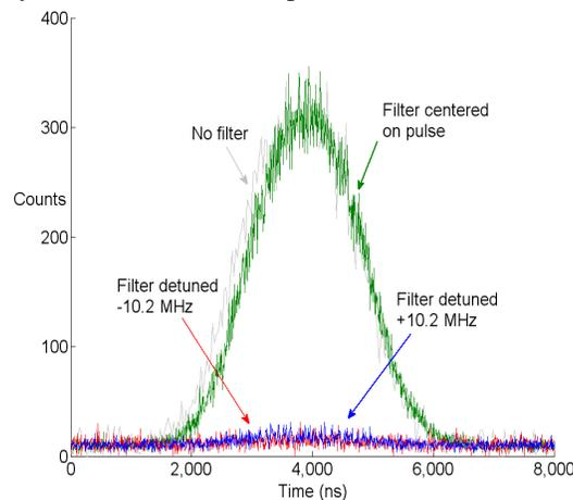
Fig. 3. Time-binned photon counts of short pulses with filter tuned to the wavelength of the light (green) and detuned by  $\pm 10.2$  MHz (blue/red). An unfiltered reference pulse (gray) shows that the filter does not significantly alter the temporal shape of the transmitted field. The slight delay of the filtered pulse compared to the unfiltered pulse can be attributed to the group velocity delay from the opening of a narrow transparency window.
