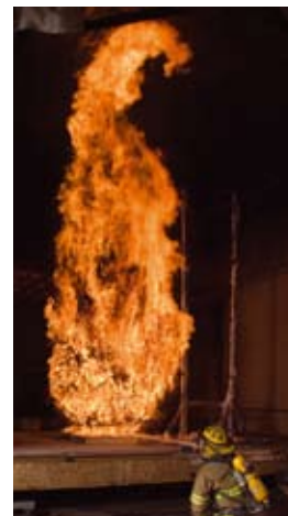
BFRL conducts experiments of burning trees in order to validate predictions of heat fluxes and heat release from simulated trees using the Wildland-Urban Interface Fire Dynamics Simulator (WFDS). WFDS is a physics based numerical modeling approach which includes all modes of heat transfer (convection, conduction, and radiation).
