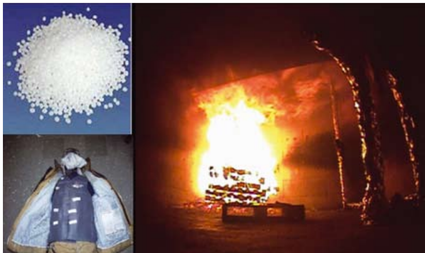
Raw phase change granular material, instrumented vest with embedded reactive cooling system, and full-scale fire exposure test.
