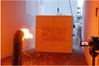
NIST Dragon unleashing a firebrand attack on a structure installed at BRI's FRWTF in Japan.
