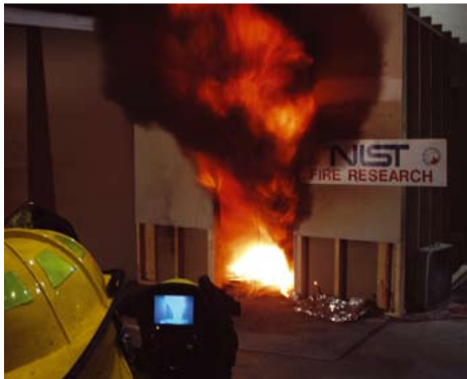
Firefighter views the opening to a furnished room with a thermal imager as the compartment flashes over
