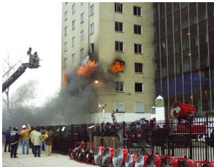
Positive Pressure Ventilation Fire Experiments conducted in 16-story residential structure with Chicago Fire Department.
