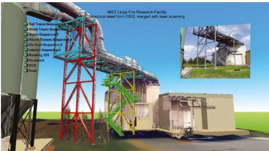
BFRL is developing methods and metrics for combining 3D imaging and building information modeling (BIM) to improve construction productivity and enable automated construction control. This image shows the combination of technologies as applied to the NIST Large Fire Research Facility.
