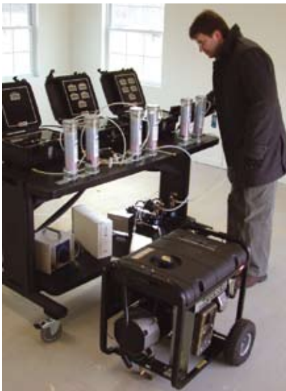
BFRL researcher Steven Emmerich adjusts a multi-gas analyzer that will measure carbon monoxide, oxygen, carbon dioxide and hydrocarbons concentrations produced by such a generator located, against safety advice, in a garage.
