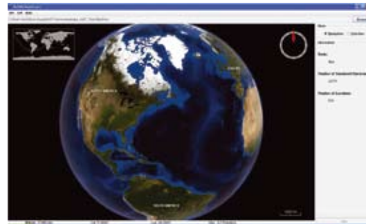
Image of the Graphical User Interface of NIST's SLOSH MapXtract program. SLOSH MapXtract is a map-based program used to extract wind speed and storm surge data and compute their joint probability for specific locations along the U.S. coastal regions.
