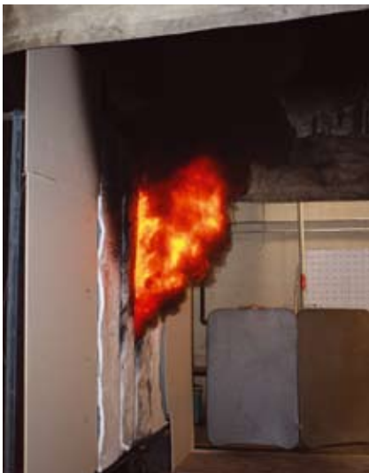
Image of a underventilated compartment fire with flames and smoke billowing out the doorway. This is typical of these types of fires and produces an environment in which it is quite difficult to make good measurements.
