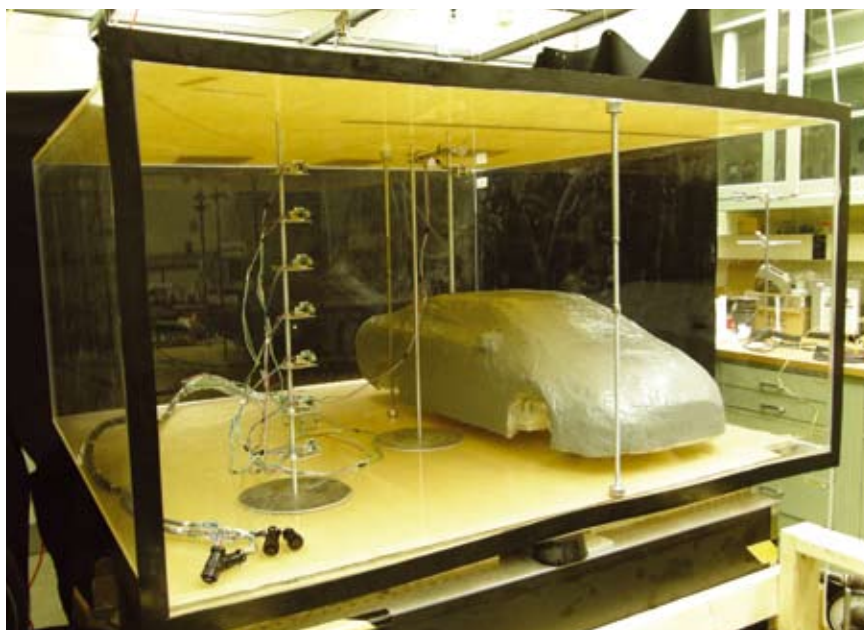
Reduced-scale garage constructed of poly(methyl methacrylate) to study the release and dispersion of helium (used as a hydrogen surrogate).
