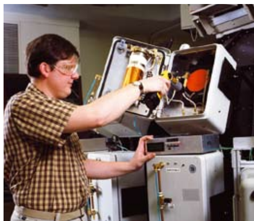
BFRL researchers are exposing NPM specimens on the NIST Simulated Photodegradation via High Energy Radiant Exposure (SPHERE).
