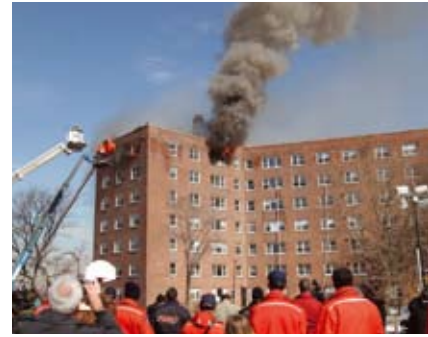
BFRL fire protection engineers use an abandoned New York City brick high-rise as a seven-story fire laboratory to better understand the fast-moving spread of wind-driven flames, smoke and toxic gases through corridors and stairways of burning buildings.
