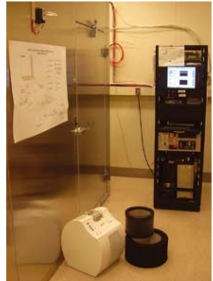
Full-scale test chamber (32 m 3 ) and the environmental and tracer gas control and monitoring systems used for testing of gaseous air cleaners, high-efficiency particle air cleaners and method development. A portable gaseous air cleaner with filters is shown in front.
