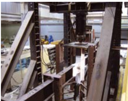
Full-scale testing of a steel beam-column assembly undergoing large displacement.
