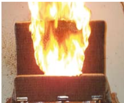
No flame penetration through barrier fabric after 6 min, whereas foam is significantly contributing without the barrier fabric after only 90 seconds.
