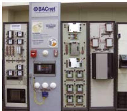
The NIST Virtual Cybernetic Testbed, a whole-building emulator used for a variety of integrated building system research activities.
