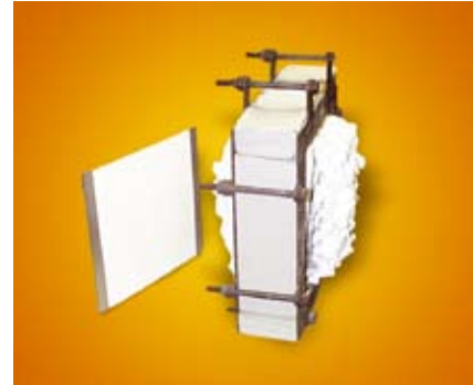
Specimen of a commercial intumescent coating prior to and after testing in the slug calorimeter high temperature experimental setup.
