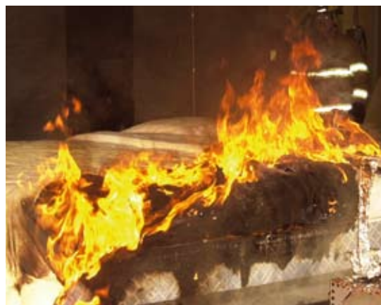
BFRL works with the U.S. mattress industry to develop the technical underpinnings for a mattress/foundation standard that would serve as the basis for limiting the consequences of residential bed fires.
