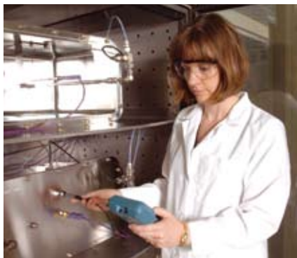
BFRL's small chamber test facility is being used to assess the performance of a reference material for building product VOC emissions testing.
