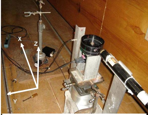
Figure 7. Rotating disk installation and coordinate system.
