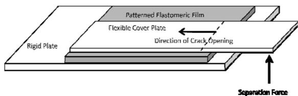
Figure 1. Schematic of the cantilever plate experiment.
