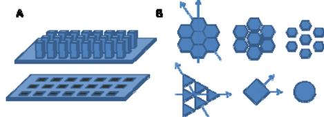
Figure 2. (A) Schematic of positive and negative pattern of square pillars. (B) Schematic array in which size and spacing of pillars is varied; two directions of crack opening are indicated by arrows.
