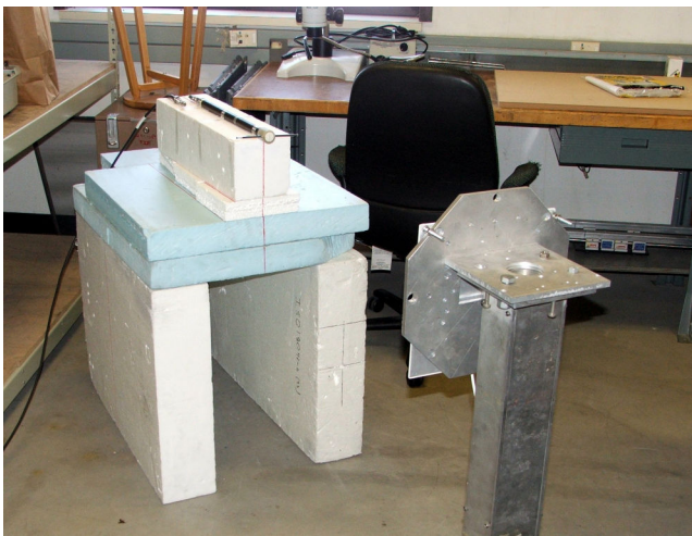
Fig. 6. The measurement setup in the reverberant storage environment under test. This room's ceiling, walls, and floor are constructed of steel-reinforced concrete. There is a large window facing outdoors above the frame, a large workbench and wall to the rear, and well-organized shelving containing test equipment on the right and left.
