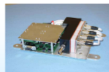
Miniaturized MultiParameter Smart Space Fire Detection System: 4 Chemical Sensors, physical sensors, and circulation pump
