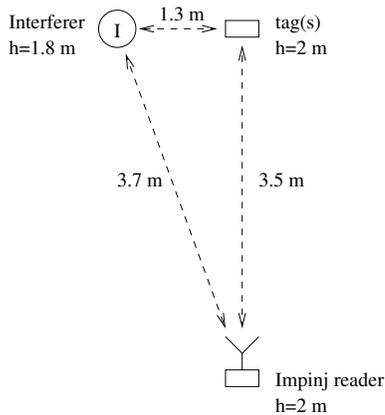
Fig. 1. Communications device illuminating RFID reader antenna
