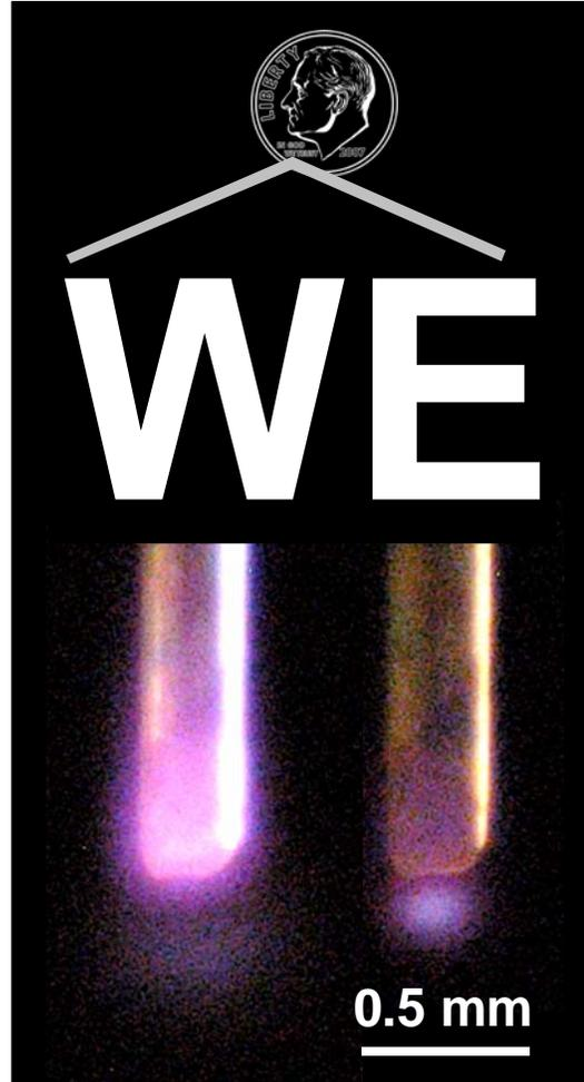
Fig. 1. Color images of hydrogen flames at their quenching limits burning in air (left) and oxygen (right).
