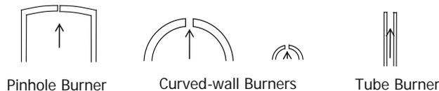
Fig. 1. Schematics of the present round-hole burners. Arrows show the fuel flow direction. Burner dimensions are given in Table 2.
