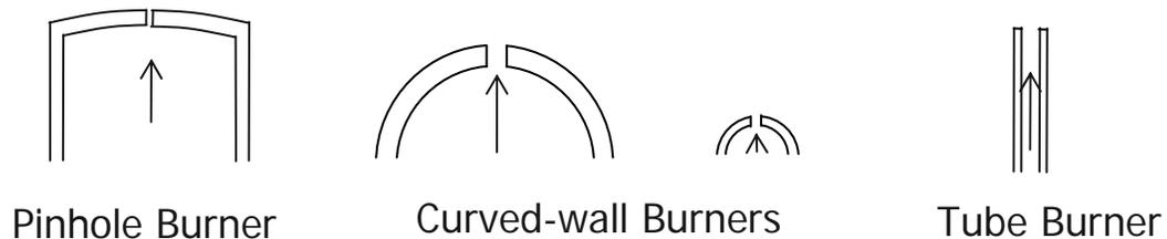
**Figure 2.1 Burners used to find quenching limits. Inside diameters for pinhole burners were mm. Inside diameters for curved-wall burners were mm (small tubes) and mm (large tubes). Tube inside diameters were mm.**
