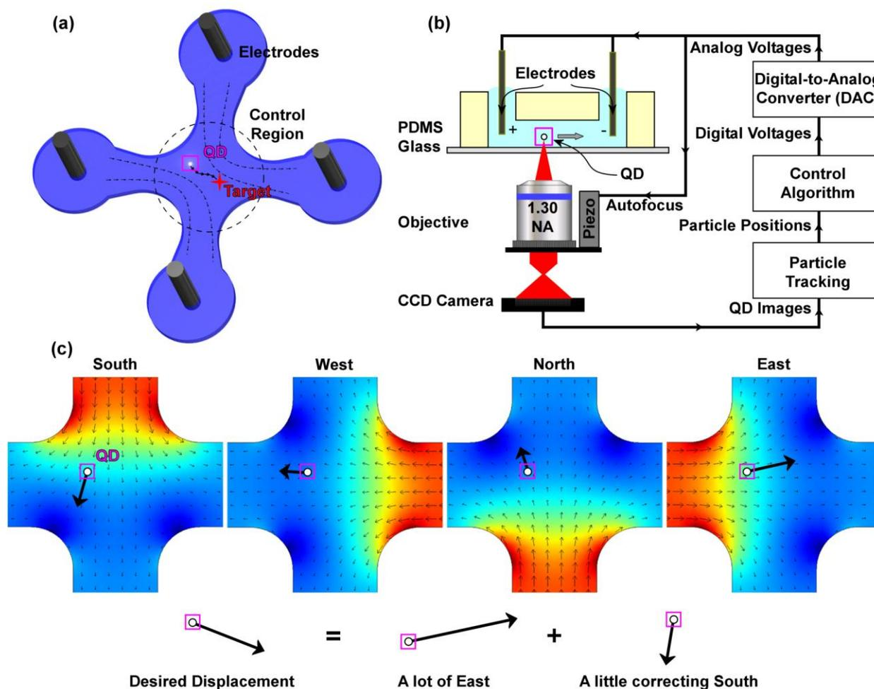
**FIGURE 1.** Experimental setup and control principle. (a) Schematic of our microfluidic device structure for 2D control of nanoparticles. An intersection between two microfluidic channels forms the control chamber of the device. Electrodes positioned in the fluid reservoirs actuate flow electroosmotically, while feedback is used to correctly move the nanoparticle to its target location. (b) Illustration of the optical and electronic setup for tracking and feedback control of QDs. A CCD camera
