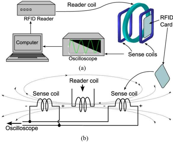
Fig. 3. (a) Measurement system for measuring the energy at carrier harmonics in RFID cards. (b) Illustration of near-field nature of an ISO 14443 transaction. We use two symmetrically placed sense coils on both sides of the reader coil to detect changes in the electromagnetic field at the same distance that the RFID card is located. We subtract the measured signal from one sense coil from the other so that we may cancel to first order the reader field in the absence of an RFID card.
