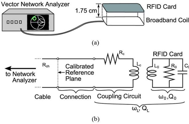
Fig. 1. Measurement system for measuring resonance in RFID cards. (a) Coupling with RFID card (b) Equivalent circuit.
