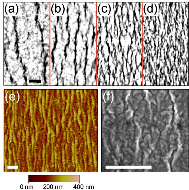
FIG. 2 (color online). Optical micrographs of membrane wrinkling ( $L = 130$  nm,  $c = 3.5 \mu\text{g cm}^{-2}$ ) for  $\epsilon =$  (a) 2.5%, (b) 5%, (c) 10%, and (d) 20%. (e) AFM and (f) SEM images reveal the complex topography of wrinkling at smaller length scales ( $\epsilon = 5\%$ ). The scale in each image is  $5 \mu\text{m}$ .
