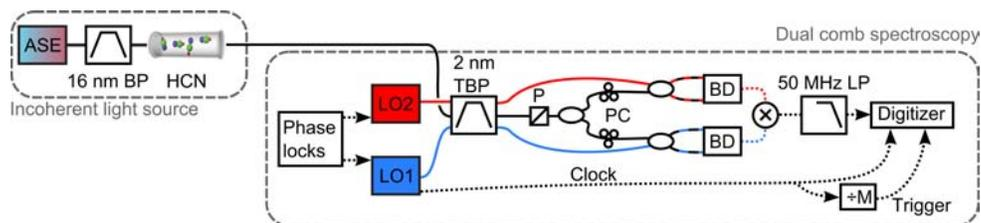
Fig. 1: Setup to measure the spectrum of an incoherent source with high frequency accuracy by sampling the spectrum in time with two asynchronous frequency combs. 16 nm BP: 16 nm wide bandpass, TBP: tunable BP, P: polarizer, PC: polarization controller, BD: balanced photodetector, LP: lowpass,  $M$ : number of pulses per frame, LO: local oscillator (frequency comb). Solid lines are fiber optic paths, dotted lines are electrical paths.
