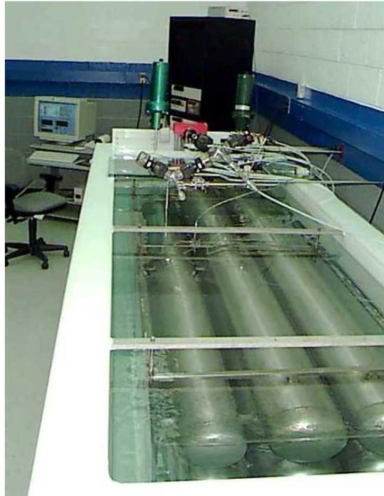
**Fig. 3** The temperature controlled 678 L collection volume.
