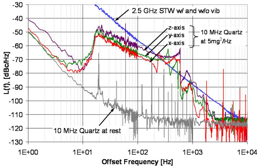
Figure 4. PM noise of the 2.5-GHz STW oscillator is shown in the topmost straight, smooth plot. The 10-MHz quartz oscillator is shown in the bottommost plot. Also shown are the PM noise plots when both oscillators are subject to 20 Hz to 600 Hz random vibration, rms level of 5 mg<sup>2</sup>/Hz. Note the dramatic increase in noise in the quartz oscillator, while no change occurs in the STW oscillator.
