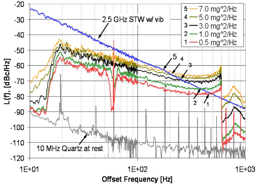
Figure 6. PM noise of free-running oscillators under vibration along the z-axis. Vibration sensitivity of each oscillator causes the optimum PLL BW at  $f_{\text{cross}}$  shown by arrows to depend on vibration level. A random vibration is applied between  $20 \text{ Hz} \leq f_v \leq 10 \text{ kHz}$ .
