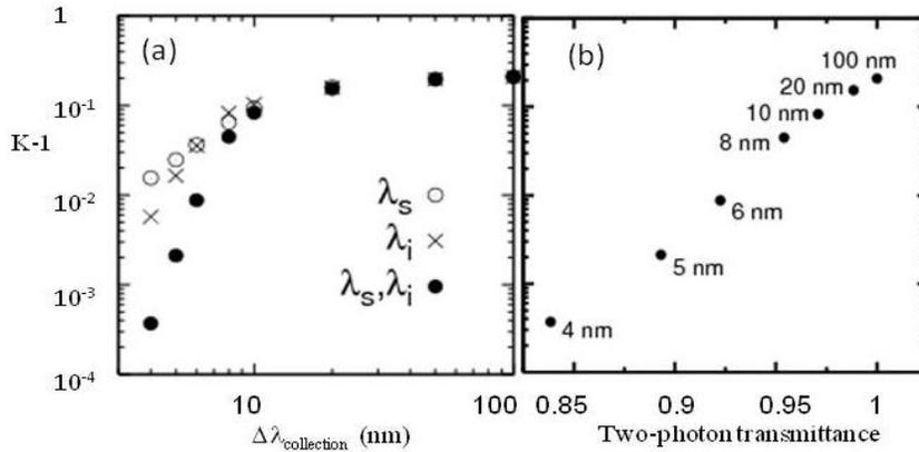
Fig. 6. (a) Degree-of-factorization of photon pairs as a function of spectral filter bandwidth, filtering only the signal, only the idler, or both. (b) Degree-of-factorization and two-photon transmittance as a function of collection bandwidth, filtering both the signal and the idler.
