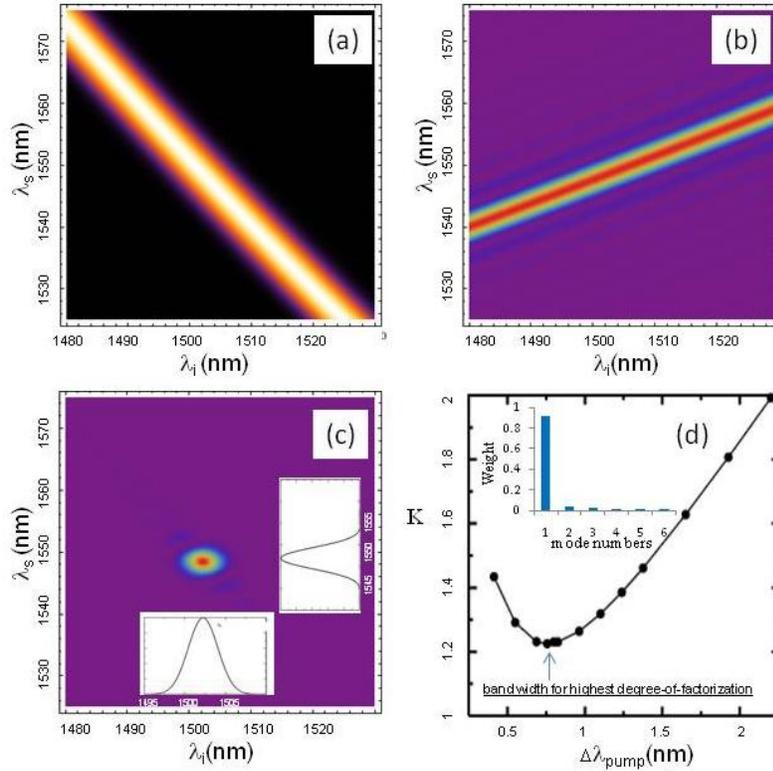
Fig. 5. Normalized spectral intensity profiles for the pump (a), phase-matching sinc-function (b), and two-photon joint spectrum (c), at the condition of the optimized pump bandwidth for the highest degree-of-factorization of two-photon joint spectrum. Insets in (c) are lineout across the center. (d) Degree-of-factorization of photon pairs as a function of the pump bandwidth. Inset in (d) is the mode distribution in the Schmidt decomposition with the optimized pump bandwidth.
