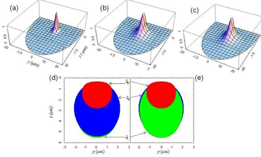
Fig. 2. Normalized transverse electric field amplitude profile for fundamental modes, (a)  $\lambda_p=764$  nm, y-polarization; (b)  $\lambda_i=1506$  nm, y-polarization; (c)  $\lambda_s=1550$  nm, z-polarization. (d)(e) Contour plots at FWHM of (a)(b)(c).
