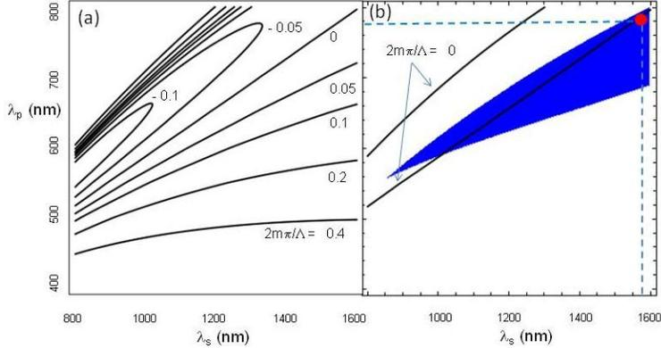
Fig. 4. (a) Sample contours for phase-matched down-conversions with different groups of pump and signal wavelengths, each group has a certain spatial harmonic frequency. (b) Shaded spectral region of interest. The red dot corresponds to the phase-matched down-conversion at  $\lambda_p = 764$  nm,  $\lambda_s = 1550$  nm and  $\lambda_i = 1506$  nm. See text for detail.
