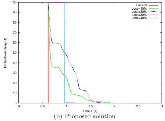
**Fig. 11** MIH handover signaling delay distribution for various packet losses in MN initiated handovers
