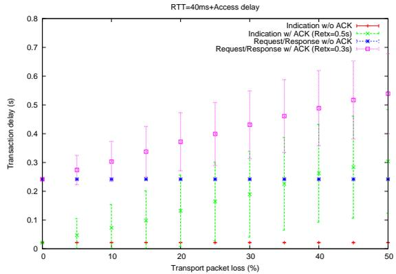
(a) Impact of packet loss on the transaction delay
