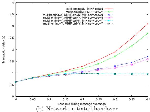
**Fig. 10** Impact of the packet loss on the MIH handover signaling delay
