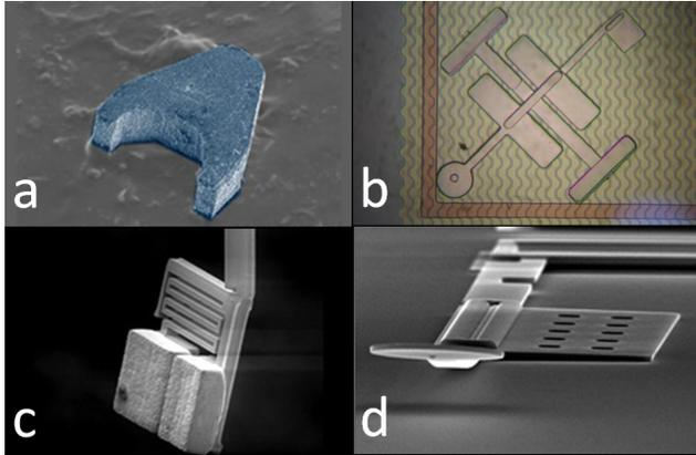
**Figure 2** Various microrobots that have been demonstrated in previous competitions: a) hard magnet microrobot (Carnegie Mellon University), b) polymer-based electrostatic microrobot (Simon Fraser University), c) resonant electromagnetic microrobot (ETH Zürich), and d) electrostatic microrobot (U.S. Naval Academy).
