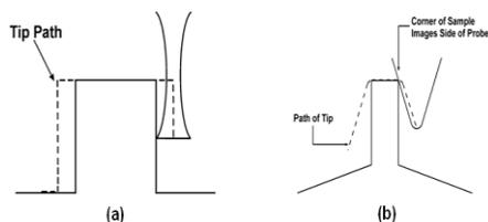
Figure 2: Schematic diagram of (a) CD-AFM tip scanning a feature, (b) conventional AFM tip scanning a feature.
