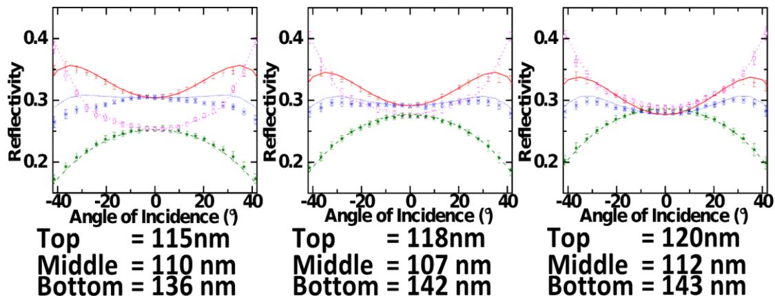
Figure 6: Experimental data and library data fits for three measurements. Top and middle critical dimensions (CDs) show good agreement with reference values.
