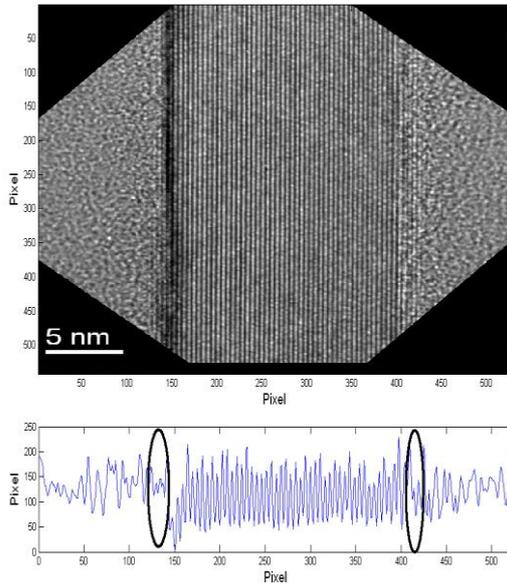
Figure 4: HR-TEM image of a SCCDRM feature. The profile is from the center of the HR-TEM image. The questionable edge locations are highlighted.
