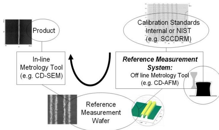
Figure1: Schematic diagram of the Reference Measurement System concept.
