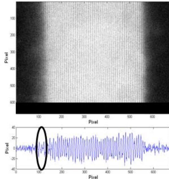
Figure 5: HAADF-STEM image of a SCCDRM feature. The profile is from the center of the HR-TEM image. The questionable edge locations are highlighted.
