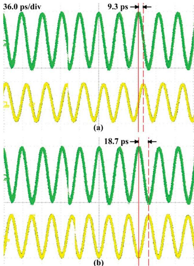
**Figure 4** Measured 90° and 180° phase shifting. [Color figure can be viewed in the online issue, which is available at [wileyonlinelibrary.com](http://wileyonlinelibrary.com)]
