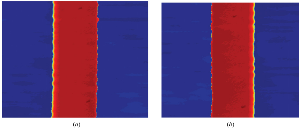
Figure 1. AFM scanning image of the linewidth sample: (a) reference image; (b) rotated image (after 180° sample rotation and 180° image rotation). The image area is about 2.3 \mu\text{m} \times 2.3 \mu\text{m} .
