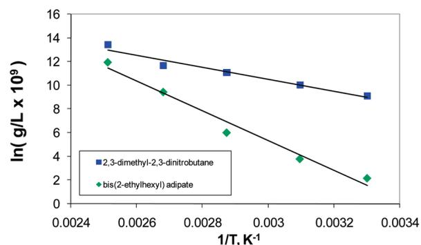
**Figure 4.** Recovered mass (grams per liter  $\times 10^9$ ) of DMNB (■) and EHA (◆), as collected with an alumina-coated PLOT column from the HS of C-4.
