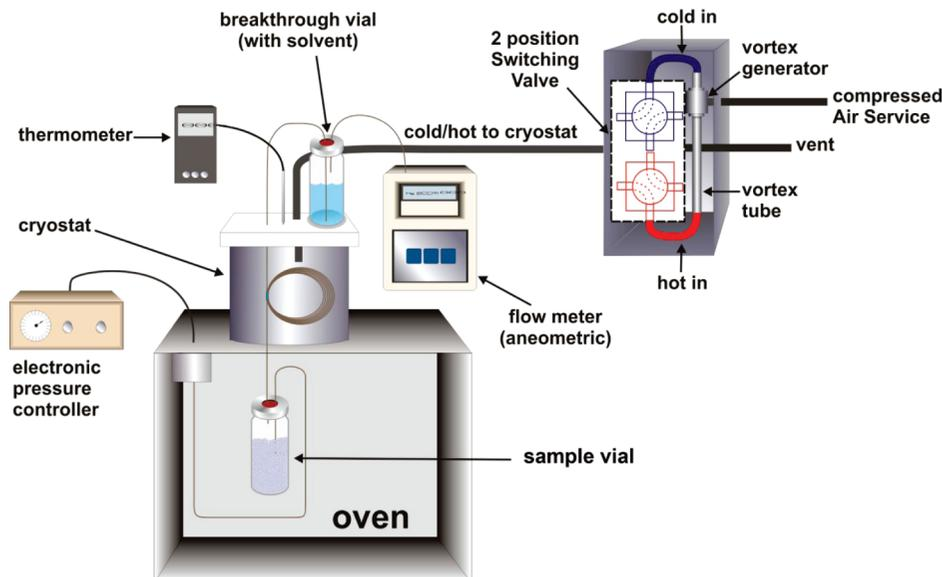
**Figure 1.** Schematic of the experimental apparatus used for quantitative and trace HS analysis with an adaptation of cryoadsorption.
