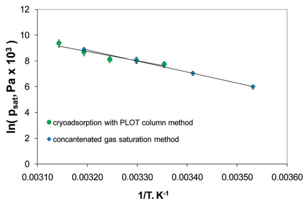
**Figure 8.** Vapor pressure ( $\text{Pa} \times 10^3$ ) of  $n$ -tetradecane, as collected with an alumina-coated PLOT column from the headspace above tetradecane adsorbed onto 1 mm glass beads (●). The data is compared with vapor pressure data obtained previously by Widegren and Bruno<sup>6</sup> by use of the concatenated gas saturation apparatus technique (◆).
