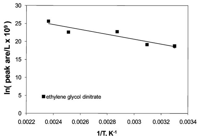
**Figure 7.** Normalized peak area (per liter  $\times 10^9$ ) of EGDN, as collected with an alumina-coated PLOT column from the HS of detcord.
