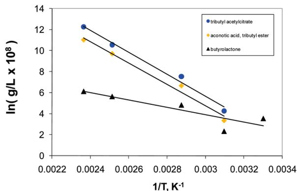
**Figure 5.** Recovered mass (grams per liter  $\times 10^8$ ) of tributyl acetylacrylate (●), tributyl aconitate (◆), and  $\gamma$ -butyrolactone (▲) as collected with an alumina-coated PLOT column from the HS of Detaflex (Flex-X).
