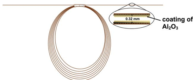
**Figure 2.** Schematic of the porous layer open tubular (PLOT) column used as a cryoadsorber trap. The PLOT column is coated with alumina, is approximately three meters long, and is coiled at a 3 in. diameter to allow the column to be housed in the cryostat chamber. (See Figure 1.)
