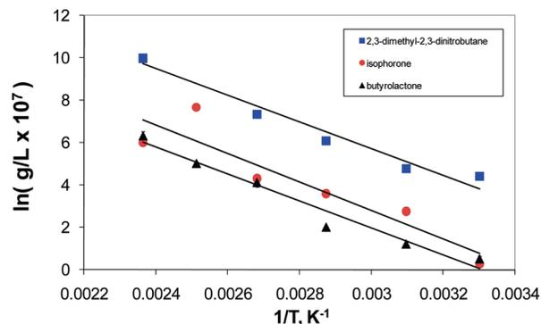
**Figure 3.** Recovered mass (grams per liter  $\times 10^7$ ) of DMNB (■), isophorone (●), and  $\gamma$ -butyrolactone (▲) as collected with an alumina-coated PLOT column from the headspace of Semtex-1A.
