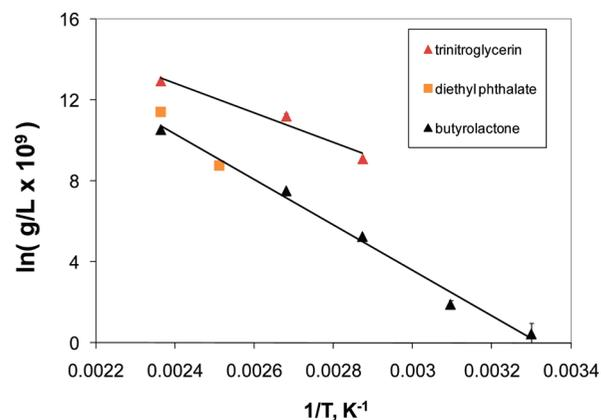
**Figure 6.** Recovered mass (grams per liter  $\times 10^9$ ) of nitroglycerin (red ▲), diethyl phthalate (■), and  $\gamma$ -butyrolactone (black ▲), as collected with an alumina-coated PLOT column from the HS of detcord.
