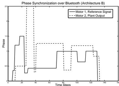
Fig. 3. Tracking control using a preliminary proportional derivative controller on architecture B (sensors and actuator communicating over a wireless Bluetooth channel). Latency and jitter in Bluetooth communication degrades control performance
