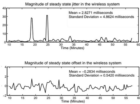
Fig. 4. Time synchronization over IEEE 802.11g wireless link using NTP. Synchronization was performed on 100 EDA nodes from simulation. Results show a mean jitter of 2.8 milliseconds.
