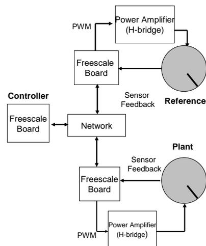
Fig. 1. A schematic of the testbed showing plant, controller boards and network components
