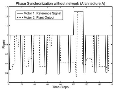
Fig. 2. Tracking control using a preliminary proportional derivative controller on architecture A (sensors and actuator hardwired to controller). Uncertainty in plant dynamics makes it difficult to achieve good tracking
