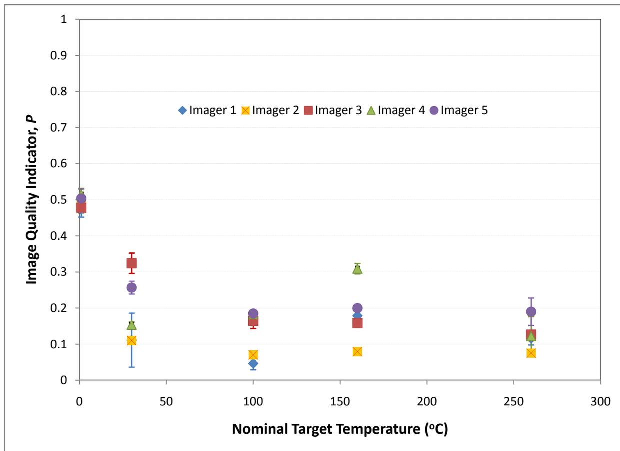
**Figure 14.** Thermal Sensitivity ( $TS$ ) plotted in terms of the image quality indicator,  $P$ . The uncertainty expressed in these test measurements is a combination of Type A (statistical) and Type B (other), with a coverage factor of 2 resulting in a 95 % confidence interval. See Section 5 for detailed uncertainty analysis.
