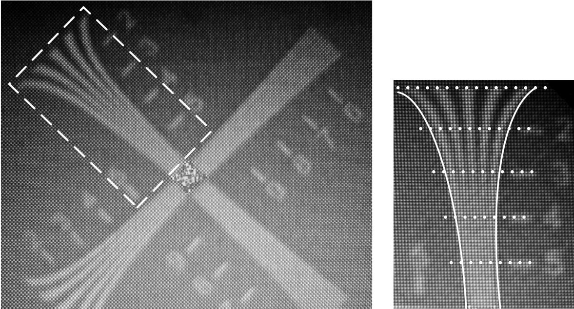
**Figure 3.** Spatial resolution image on left with a dashed box indicating the inset image on right. The ROI is between the solid white lines in the right image and the dotted lines show the position and orientation of the rows of pixels used to calculate the *CTF*.
