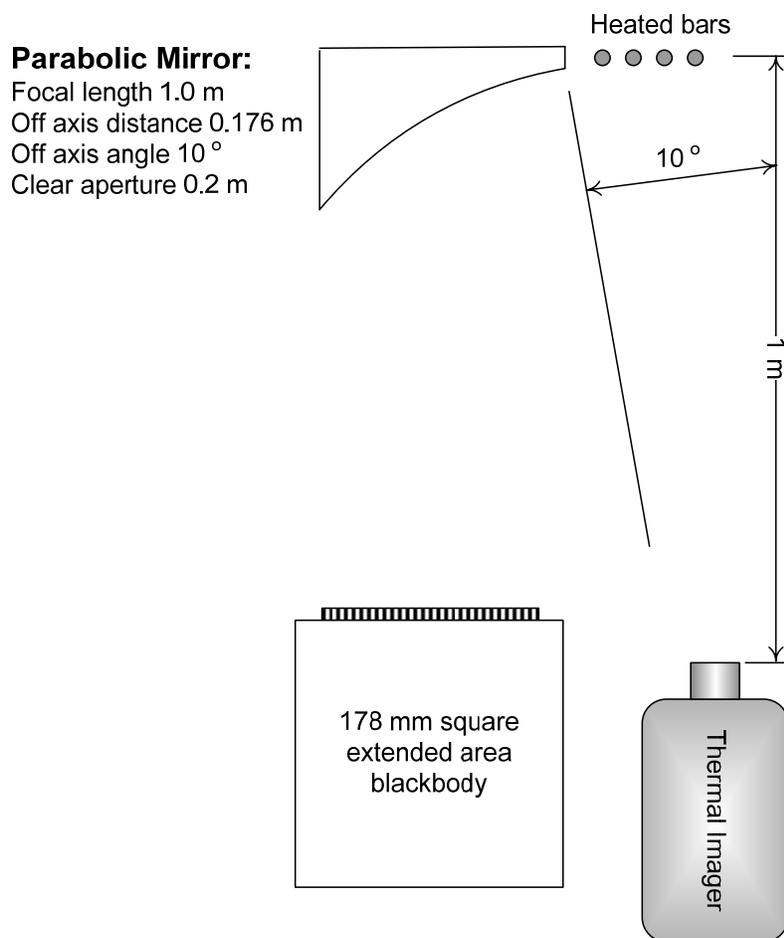
**Figure 4.** *ETR* testing configuration. The target consists of the heated bars, which appear on the side of the image, and the emitting surface of the blackbody, which appears in the center of the image.
