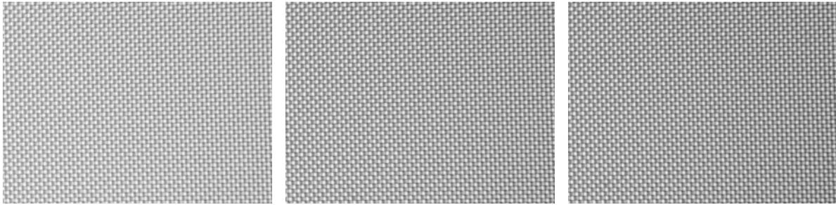
**Figure 5.** Example test images for *TS* at a nominal target temperature of 100 °C. The image on the left is of a 100.05 °C target, the image in the center is of a 100.00 °C target, and the image on the right is of a 99.95 °C target. Note that these three images may appear to be identical when viewed on a printed page.
