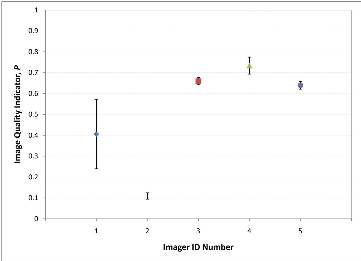
**Figure 10.** Spatial resolution ( $SR$ ) plotted in terms of the image quality indicator,  $P$ . The uncertainty expressed in these test measurements is a combination of Type A (statistical) and Type B (other), with a coverage factor of 2 resulting in a 95 % confidence interval. See Section 5 for detailed uncertainty analysis.
