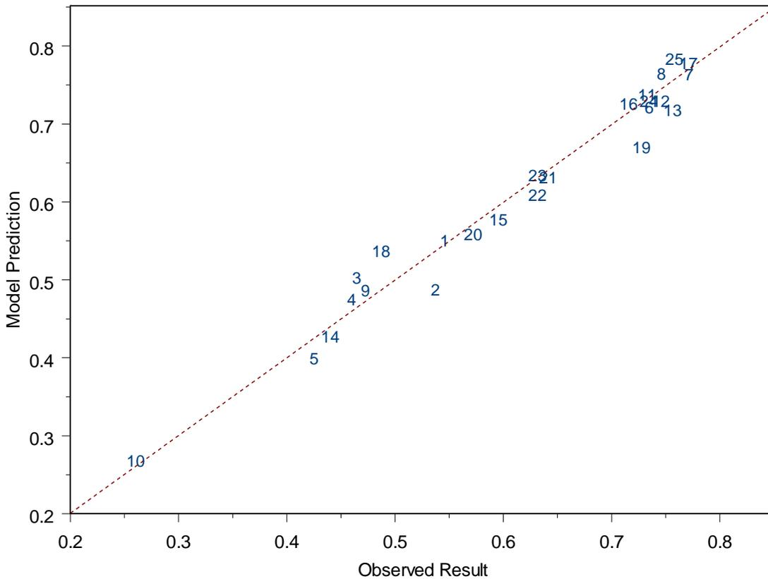
**Figure 7.** A comparison of the observed and model predicted values for the probability of successfully completing the fire hazard identification task. The plot character represents the image setting (1 to 25). A perfect correlation falls at the 45° diagonal.
