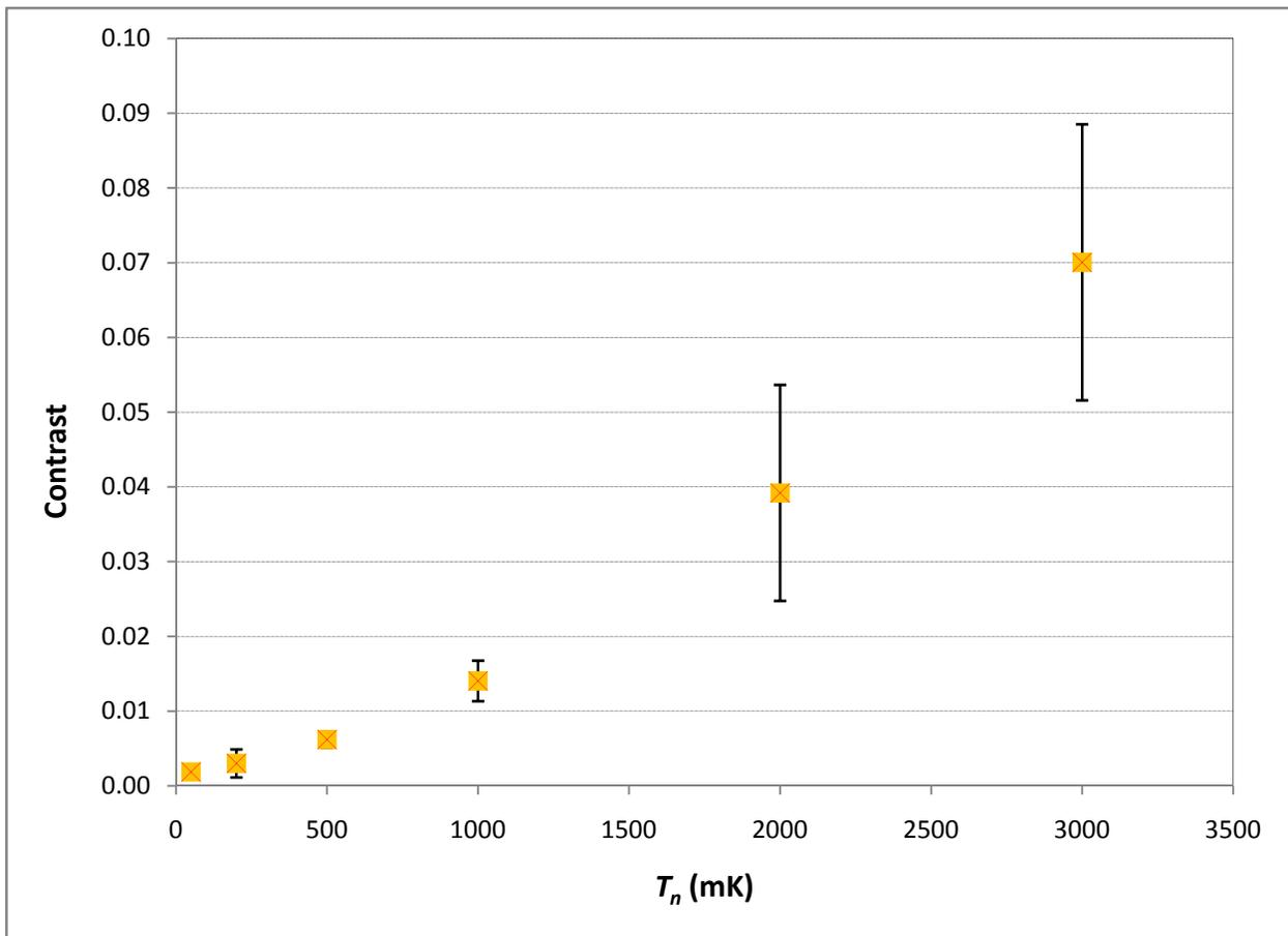
**Figure 6.** Contrast response to increasing values of  $T_n$  for the *TS* test. The nominal target temperature was 100 °C. The uncertainty expressed in these test measurements is a combination of Type A (statistical) and Type B (other), with a coverage factor of 2 resulting in a 95 % confidence interval. See Section 5 for detailed uncertainty analysis.
