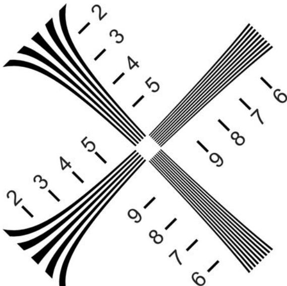
**Figure 2.** Spatial resolution thermal target. The foreground (black markings) is held at a constant temperature of 3 °C above ambient. The target size is 61 cm measured along the centerline of each of the two converging line sets.
