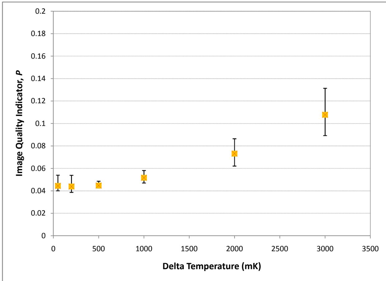
**Figure 15.** Thermal sensitivity as a function of increasing delta T ( $T_n$ ). The uncertainty expressed in these test measurements is a combination of Type A (statistical) and Type B (other), with a coverage factor of 2 resulting in a 95 % confidence interval. See Section 5 for detailed uncertainty analysis.
