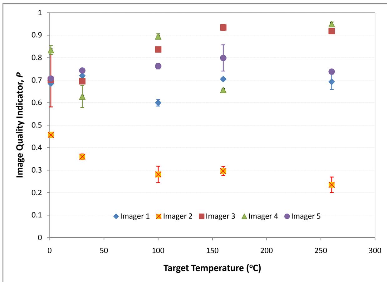
**Figure 9.** Nonuniformity ( $NU$ ) plotted in terms of the image quality indicator,  $P$ . The uncertainty expressed in these test measurements is a combination of Type A (statistical) and Type B (other), with a coverage factor of 2 resulting in a 95 % confidence interval. See Section 5 for detailed uncertainty analysis.
