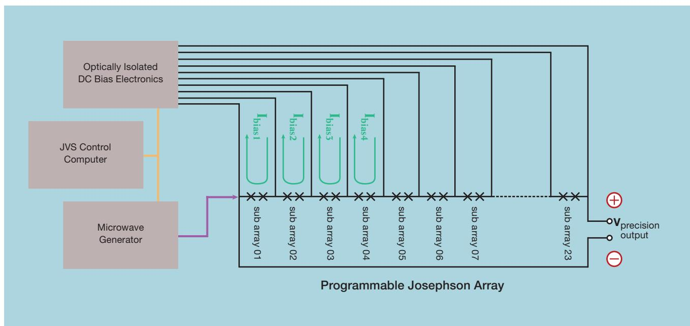
**Figure 3.** System block diagram for the new “turnkey” 10 V PJVS.
