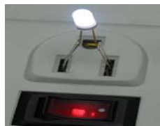
Figure 1. Photo of an AC LED plugged into the mains supply
