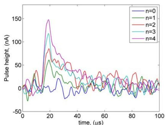
**FIGURE 5.** Detector response to 850 nm (1.46 eV) photons. The pulses correspond to zero-, one-, two-, three-, and four-photon events. The measured (1/e) decay time is ~ 20  $\mu$ s.
