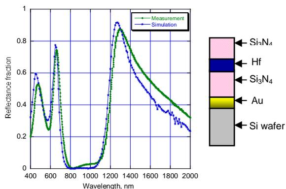
**FIGURE 3.** Optical structure for Hf optimized TES devices at 850 nm. The plot shows good agreement between predicted reflectance of the stack (simulation) and reflectance measurement of the stack (measurement).
