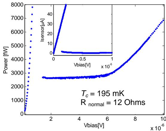
**FIGURE 1.** Power and current (inset) as a function of voltage bias for  $25 \mu\text{m} \times 25 \mu\text{m}$  Hf TES. Below  $5 \mu\text{V}$  the sensor is self-biased.
