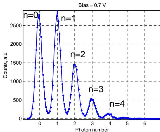
**FIGURE 4.** Pulse-height distribution of a pulsed laser source measured with the Hf TES embedded in the optical cavity. The source was 10 ns wide pulses of 850 nm laser light at a repetition rate of 10 kHz and containing an average photon number of  $\mu \sim 1.06$ .
