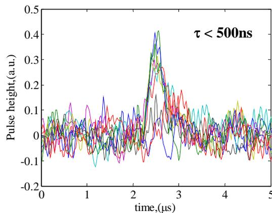
**FIGURE 2.** Hafnium (bare) device response to 850 nm ( $1.46 \text{ eV}$ ) photons. The measured  $(1/e)$  decay time is  $\sim 500$  ns.
