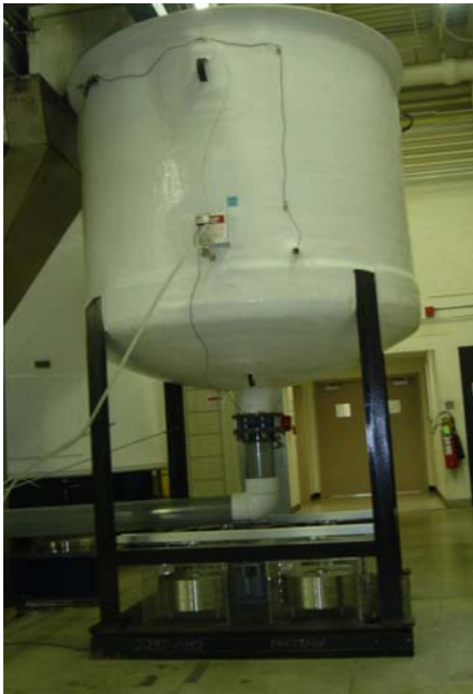
Figure 2. Collection tank resting on scale. Calibration weights are visible near floor.
