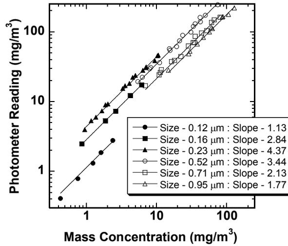
Fig. 2. Mass concentration versus photometer reading for DOP aerosols.
