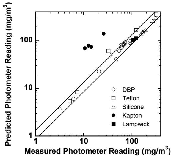
Fig. 4. Comparison of predicted photometer readings to measured readings for SAME experiment smokes. Most predictions fall within a range of  $\pm 25\%$  deviation from measured with the notable exception of Kapton.
