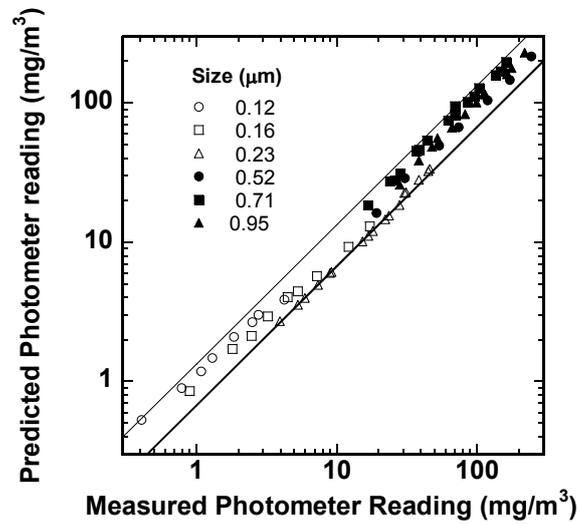
Fig. 3. Comparison of predicted photometer readings to measured readings for DOP aerosols. The lines bound a  $\pm 33\%$  spread between the measured and predicted values.
