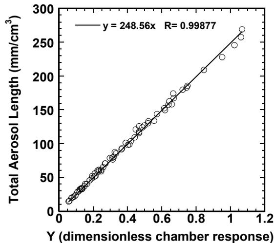
Figure 1. Total aerosol length versus Y for DOP aerosols.
