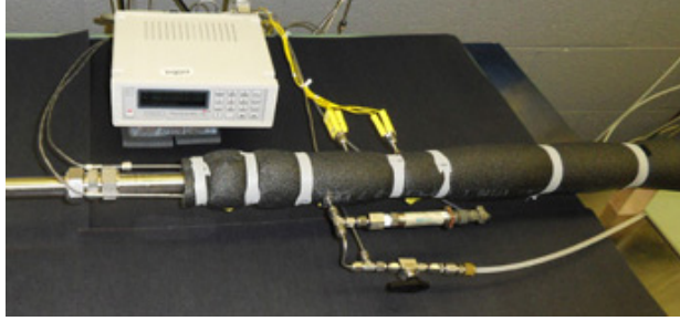
Fig. 4 A photograph of the CFV test section for the blow-down tests.
