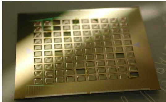
**FIGURE 1.** Prototype of a 100 pixel MUSTANG array. This array is very similar to the array that we are modeling. The substrate is a 275  $\mu\text{m}$  thick Si wafer with 500 nm thick SiN membranes. Each pixel is 2 mm by 2 mm and the pixel to pixel pitch is 2.5 mm. The pixels have MoCu bilayer TES thermometers with Nb wiring and a PdAu mesh to absorb 90 GHz radiation. This prototype does not include NIS coolers, heatsinking bond pads or underside Au.
