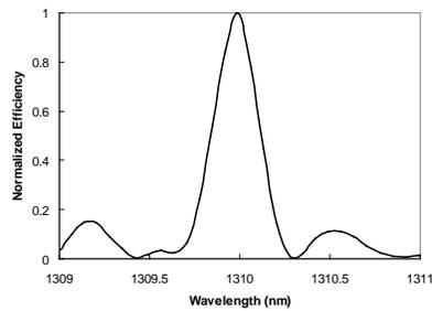
Fig. 4. The normalized detection efficiency as a function of signal wavelength, when the pump wavelength and temperature of the waveguide are fixed.
