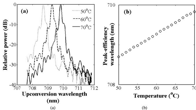
Fig. 5 (a) The normalized output spectrum of the PPLN at the different temperatures shown in inset. (b) The up-conversion wavelength peak as a function of temperature.
