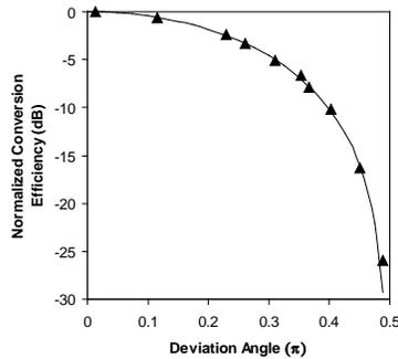
Fig. 6. The normalized conversion efficiency of the PPLN waveguide as a function of deviation angle of the input signal at 1310 nm. The deviation angle is the angle between the given polarization state and the state at which the conversion efficiency is maximized. Triangle: Measurement results; Solid line:  $\cos^2(\cdot)$  curve
