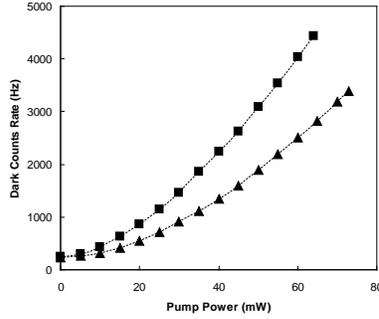
Fig. 3. The dark count rate as a function of pump power at the PPLN input. Two cases are studied: CW pump (triangle) and pulsed pump (square).
