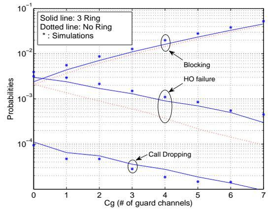
Fig. 3. Plot of blocking probability ( $P_B$ ), handoff failure probability ( $P_f$ ), and probability of dropped call due to mobility ( $P_D$ ) in modified conventional ( $K = 1$ ) and ring-based ( $K > 1$ ) queueing models.
