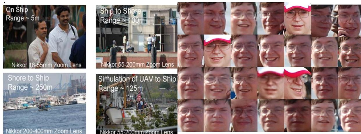
**Figure 7: Examples of face images acquired at different distances from the camera.**
