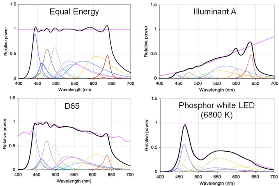
Figure 4. Spectral matching of the STLS to standard illuminants and an LED spectrum.
