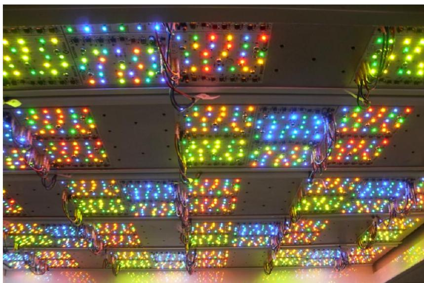
Figure 3. The six LED board types mounted on the heat sinks installed in the STLS.
