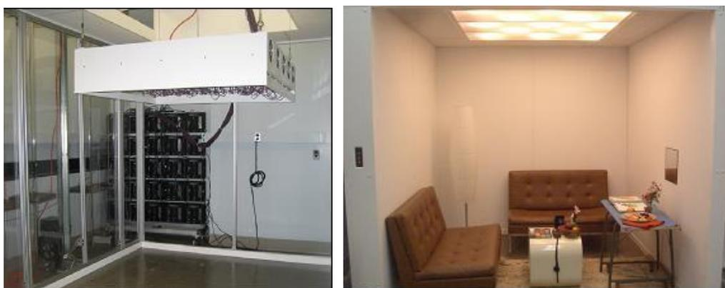
Figure 1. Left: an STLS lowered from the ceiling (with the walls of the cubicle removed). Right: one of cubicles lit by the STLS, to be used for color rendering experiments.
