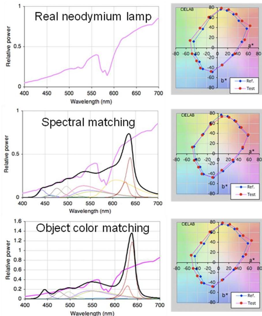
Figure 5. The spectrum of the neodymium lamp (top), the STLS spectrum using the spectral matching algorithm (middle) and the spectrum from the object color matching algorithm (bottom). The CIELAB plots show the change in chromaticity coordinates for the 15 object colors used in the CQS referenced to a blackbody.
