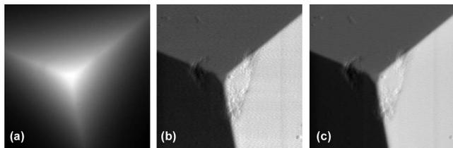
FIG. 1. (a) Topography, (b) phase, and (c) oscillation amplitude contrast images of a Berkovich diamond. Oscillation phase and amplitude are distinctly dependent on the facet being imaged. Width of field is  $2.5 \mu\text{m}$ .
