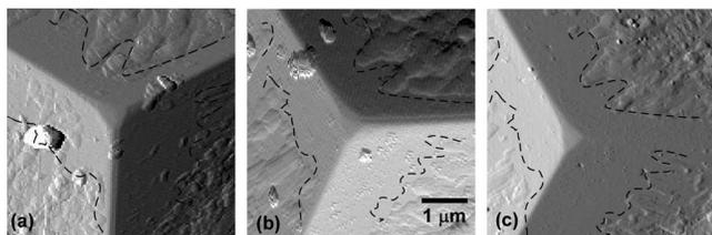
FIG. 2. Amplitude contrast images of diamond probe after (a) repeated solvent cleaning, then (b) oxygen plasma cleaning, and, finally (c),  $\text{CO}_2$  snow cleaning. The black dotted lines were drawn to roughly outline the remaining detritus in (c), then copied to (a) and (b) to show the evolution of the diamond surface.
