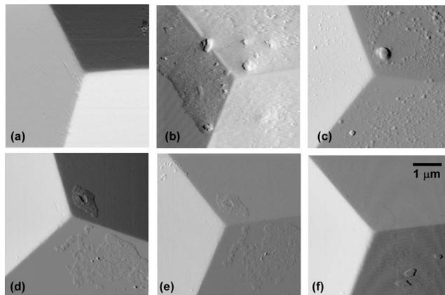
FIG. 3. Amplitude contrast images of a Berkovich diamond nanoindentation probe (a) initially clean, (b) after indentation into a fingerprint, (c) solvent cleaning, (d) snow cleaning, (e)  $\text{O}_2$  plasma+snow cleaning, and (f) after pressing into wood+snow cleaning.
