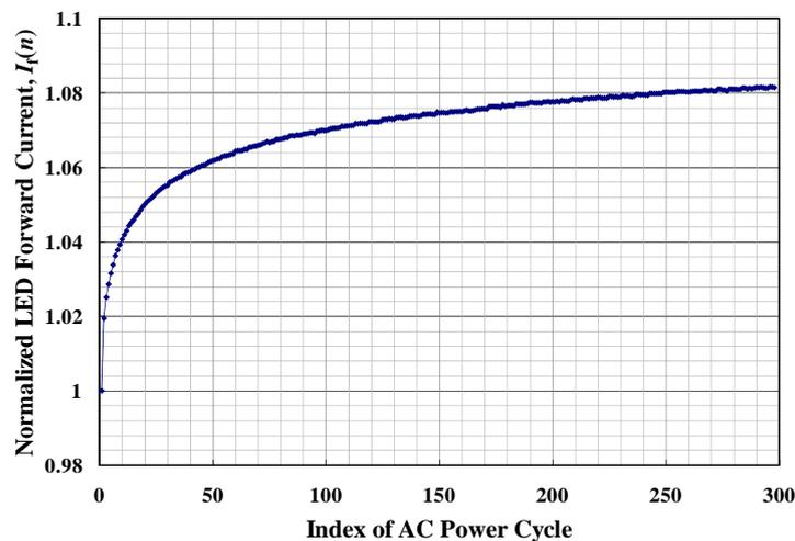
Figure 5. A heating curve of an AC LED.
