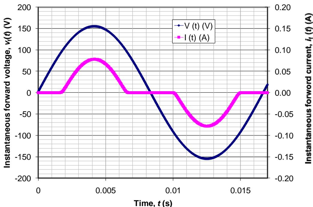
Figure 2. Instantaneous forward voltage,  $v_f(t)$ , and forward current,  $i_f(t)$ , of a 110 V AC, 60 Hz LED.
