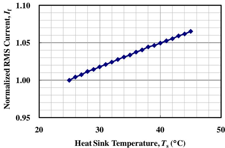
Figure 4. Relationship between the LED RMS forward current,  $I_f$ , and the heat sink temperature,  $T_j$
