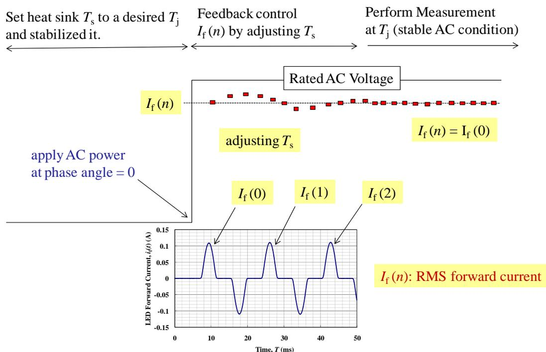
Figure 3. Principle of the simple method for measurement of AC LEDs
