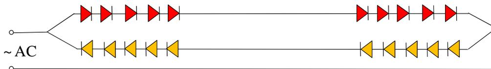
Figure 1. Illustration of the design of an AC LED
