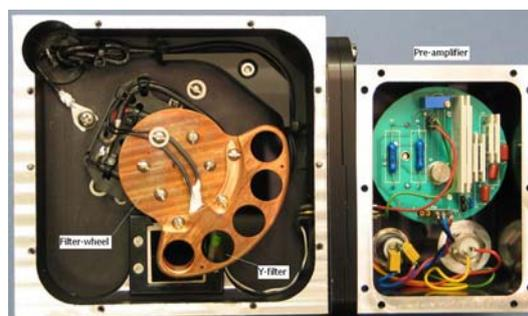
**Figure 1.** Picture of the single-element Si photodiode based colorimeter.
