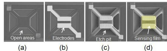
**FIGURE 1.** Steps for converting a microhotplate precursor to a functional gas-sensor.
