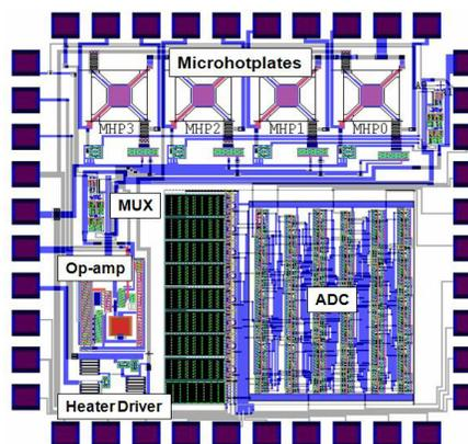
**FIGURE 4.** A layout of a 2 mm x 2 mm gas sensor system chip showing four microhotplates, an 8-bit ADC, an op-amp, a MUX, and a heater driver.
