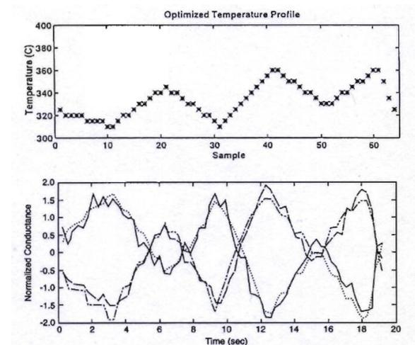
**FIGURE 3.** (top) Temperature program sequence. (bottom) Methanol and ethanol response to temperature program.
