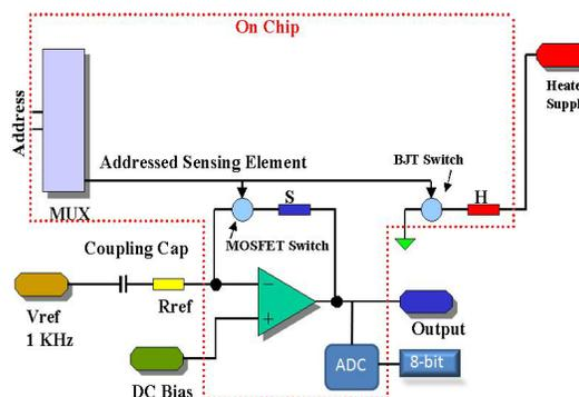
**FIGURE 5.** Schematic diagram of gas-sensor system of the gas-sensor chip layout shown in Fig. 4. Only the circuits associated with one of the four microhotplate heaters are shown.
