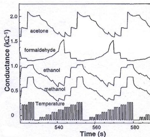
**FIGURE 2.** Shows response curves from a microhotplate-based, palladium-doped, tin-oxide gas sensor when exposed to different gas species with temperature-programmed sensing.
