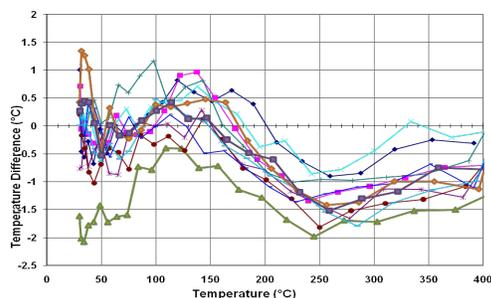
**FIGURE 6.** Differences between the microhotplate temperatures measured with platinum-rhodium thermocouple and microhotplate thermal resistance at 11 different times during a period of 3 months.
