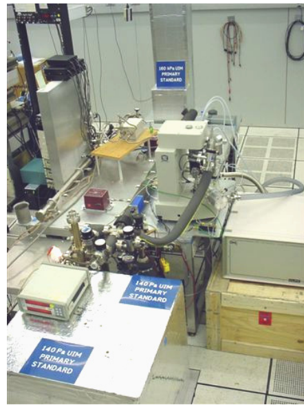
Fig. 3. Shown above is an FPG unit under test at NIST being compared to the 140 Pa Oil UIM and the 160 kPa mercury UIM pressure standards.
