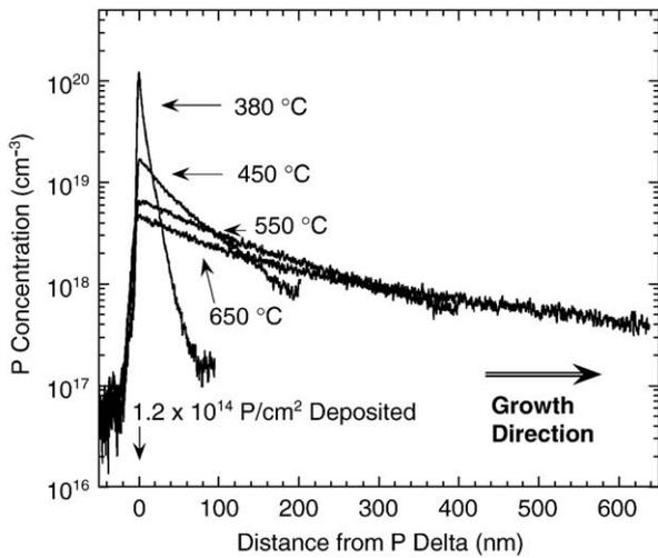
Fig. 1. SIMS atomic concentration profiles of P resulting from a delta layer deposited at "0" followed by undoped Si deposited at temperatures between 380 °C and 650 °C.
