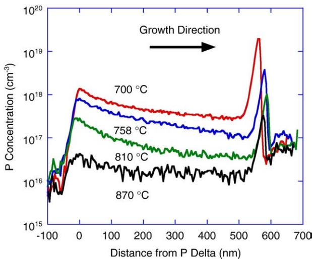
Fig. 2. SIMS atomic concentration profiles of P resulting from a delta layer deposited at "0" and undoped Si deposited at temperatures between 700 °C and 870 °C. Room temperature Si was deposited to trap the surface P at the end of growth.
