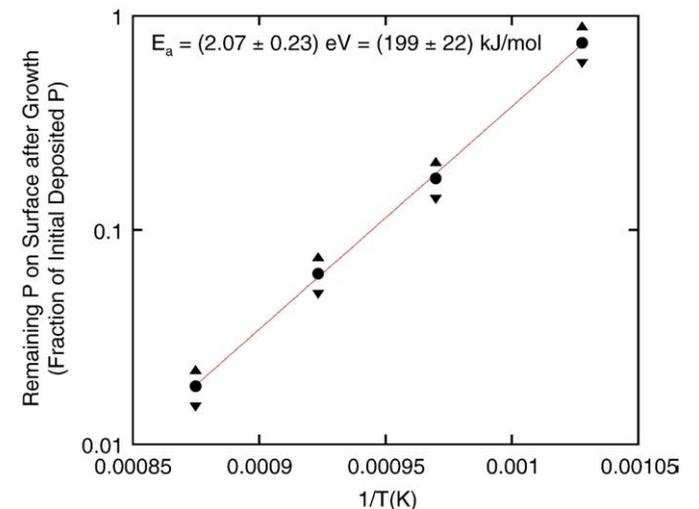
Fig. 4. Determination of the activation energy for P evaporation from the Si surface. Error bars (triangles) represent ±20% estimated relative uncertainty in atomic concentration measured by SIMS.
