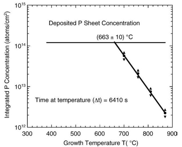
Fig. 3. Total P in the sample including the P trapped at the surface. Δ*t* is the total time at the growth temperature. There is clear evidence of P evaporating from the surface during growth. Error bars (triangles) represent ±20% estimated relative uncertainty in atomic concentration measured by SIMS.
