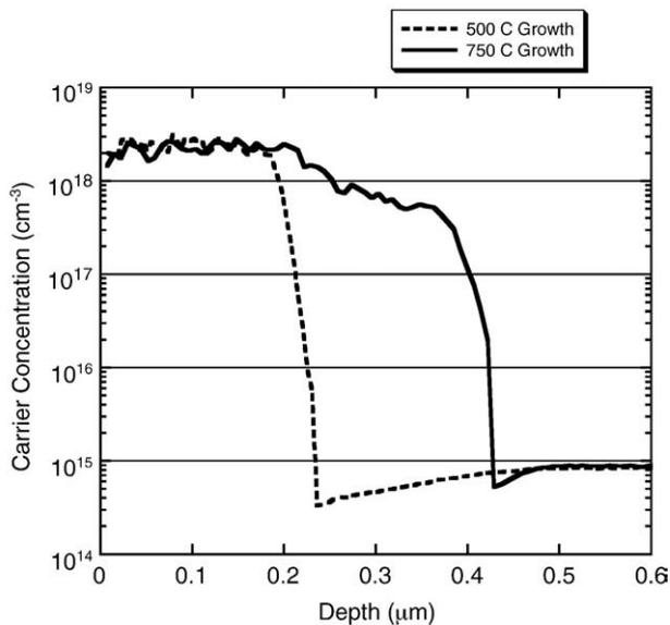
**Fig. 5.** Uniform P doping at 750 °C was obtained by using a P delta layer pre-deposition and high P flux to compensate for both surface evaporation and surface segregation. Uniform P doping at 500 °C is shown for comparison.
