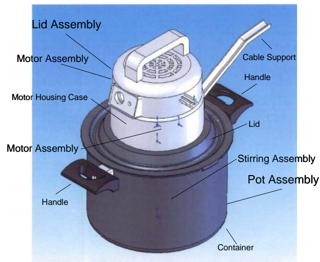
Figure 10: Automatic Pot Stirrer components [24]
