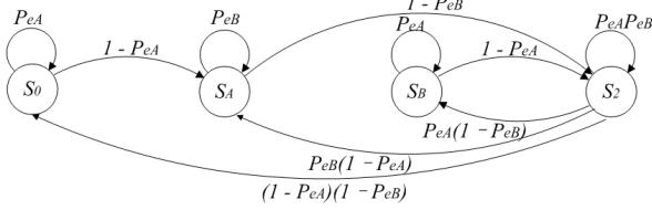
Fig. 6. Markov chain for state transitions of  $n_R$
